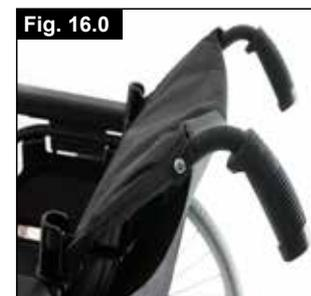
To fold the backrest, stand behind the wheelchair, press the two small levers (Fig. 16.0) positioned on each side of the backrest (just above the armrests). Fold the backrest down.
