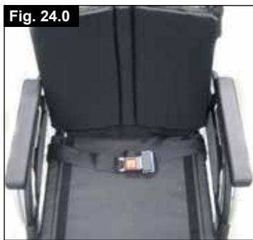
The lap belt should be fixed so that the belt sits at an angle of 45 degrees across the user's pelvis. The user should be upright and be as far back as possible in the seat when correctly adjusted. The lap belt should not allow the user to slip down in the seat. (Fig.26.0)
