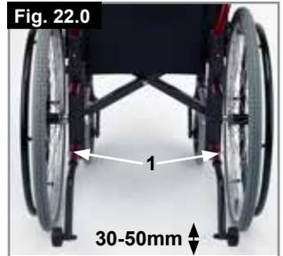
By pushing on the release button (1), the safety wheels can be set upwards or removed. There must always be a gap of between 30mm and 50mm between the tube and the ground.
